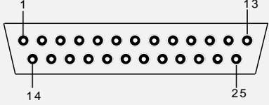
The diagram shows a 25-pin connector with two rows of pins. The top row has 13 pins, with the first and last pins labeled 1 and 13 respectively. The bottom row has 12 pins, with the first and last pins labeled 14 and 25 respectively.
