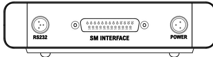
Fig 5. Rear panel view of the SC1 modules
