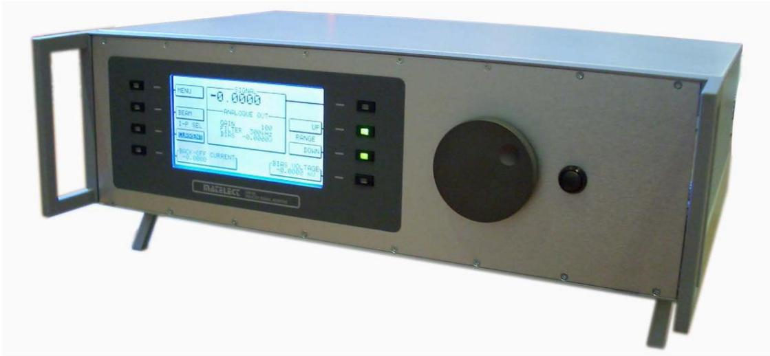
Used mainly in the EBIC mode (electron beam induced current), the ISM-6A is employed in conjunction with a scanning electron microscope to image electrically active defects in semiconductor materials and devices. Long regarded as the industry leader, the ISM series offers quantitative as well as qualitative facilities, the former enabling device parameters and materials data to be obtained. The ISM-6A builds on the original ISM-5 unit which is found in many research labs worldwide.
