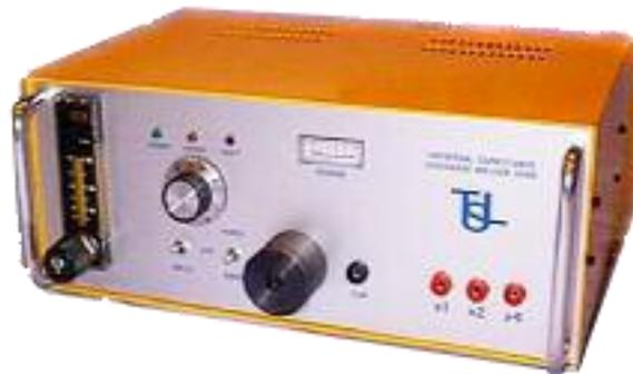
The model SR-80 thermocouple welder has been specifically chosen by Matelect for the welding of potential drop current and signal cables to the specimen under test. Using capacitance discharge as the energy for the weld, wires of up to 1.6mm diameter can easily be welded with minimum user experience.
