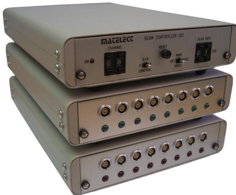
To increase the versatility of the CGM-5R crack growth monitor, Matelect developed a compact, modular signal multiplexing system designed to allow multi-point monitoring of specimens undergoing crack growth Measurements.
