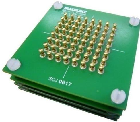
Used in conjunction with any of the Matelect PD products, this small device has 64 pins laid out in a 8 x 8 grid, two pins can be simultaneously selected allowing for a potential drop measurement to be made.
