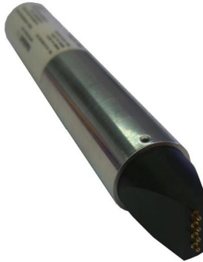
Matprobes are designed to be used with the CGM series of crack growth monitors, allowing the user to obtain crack depth data in the field without the need to provide permanent contact to a specimen. Spring loaded pins are utilised to form some or all of the contacts necessary for operation. The probes are designed to be used as handheld devices although it is possible to incorporate them into other apparatus to maintain fixed geometries (e.g. for use on a production line).
