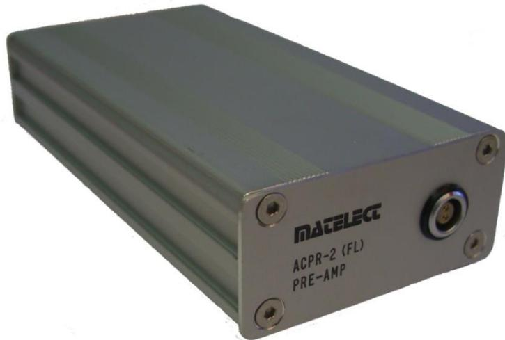
The ACPR-2 (FL) is a filtered pre-amplifier, specifically developed for use with the CGM-7 and CGM-5R. When using an induction furnace for high temperature experiments the induction coils can affect the signals of the ACPD test, therefore a filter is required to cut-out the high frequency interference. As standard these units have a 10kHz cut-off frequency, other cut-off frequencies may be available on request.
