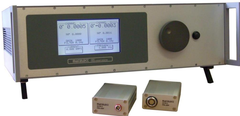
The CGM-7 is a modern microprocessor based instrument for measuring crack depth in metals undergoing materials testing. Building on the success of the CGM-5R this unit improves upon the CGM-5R specification by offering two channel operation, higher frequency and current outputs, full computer control and a variety of expansion options.
