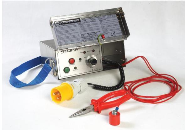
The Stork Thermocouple Attachment Unit (TAU) has been specifically chosen by Matelect for the welding of potential drop current and signal cables to the specimen under test. Using capacitance discharge as the energy for the weld, up to 24 gauge (awg) wires can easily be welded with minimum user experience.
