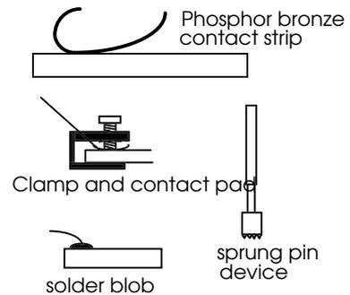
Fig 3. Suggested methods of achieving specimen contact.
